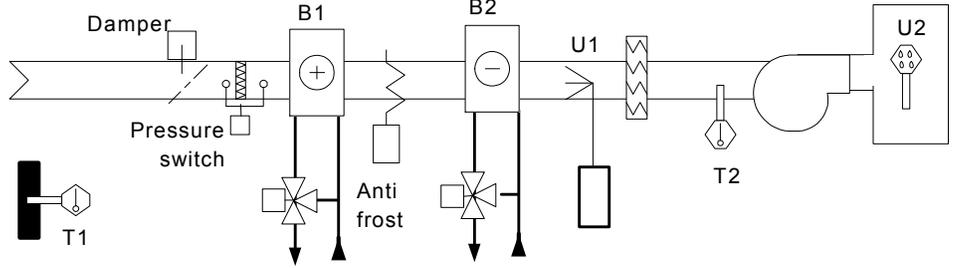
1: Primary air. 2 coils (heating, cooling), humidification. Compensated or set point adjustment of the dew point. On/Off humidifier, anti-frost thermostat. The inputs marked by ° are optional. The stroke end, if not used, must be short-circuited, in order to have a "On" value; the others must be left free.
