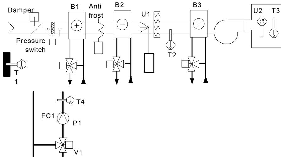
5: 4 + 2-pipe fan-coil water production. Compensated or set point control of hot water in winter; compensated or set point control of cold water through external summer/winter switch.
