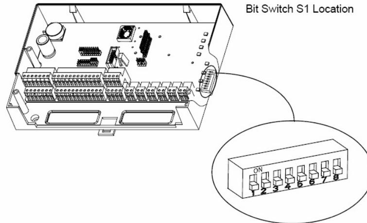
Example: to configure address 37: set switches 1, 3 and 6 to ON and the other switches to OFF position.
