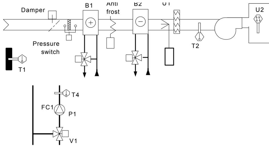
2: 1+ 2-pipe fan-coil water production. Compensated or set point control of hot water in winter; compensated or set point control of cold water through external summer/winter switch. The inputs marked by ° are optional. The stroke end, if not used, must be short-circuited, in order to have a "On" value; the others must be left free.
