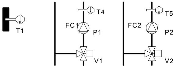
9: 4-pipe fan-coil water production. Compensated or set point control of hot water in winter; compensated or set point control of cold water. The inputs marked by ° are optional.
