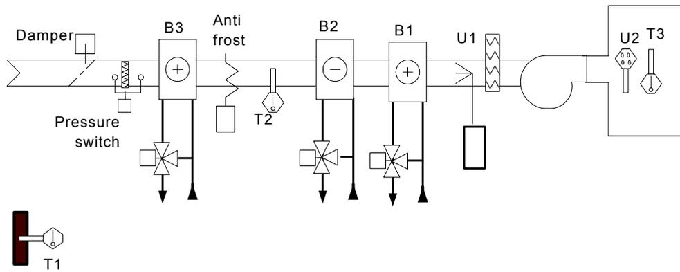
7: AHU outside air. Pre-heating, heating, cooling, humidification. Compensated or set point control of pre-heating and room temperature. On/Off humidifier. Anti-frost thermostat. Room temperature manual control (optional).
