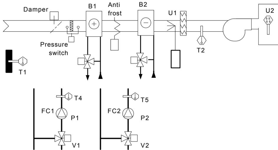
3: 1+ 4-pipe fan-coil water production. Compensated or set point control of hot water in winter; compensated or set point control of cold water.
