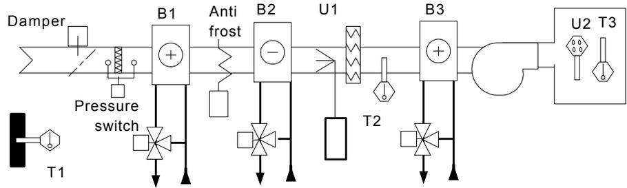
4: Primary air. 3 coils (heating, cooling, post-heating) humidification. Compensated or set point control of dew point and supply temperature. On/Off humidifier, anti-frost thermostat.
