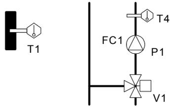
8: 2-pipe fan-coil water production. Compensated or set point control of hot water in winter; compensated or set point control of cold water through external summer/winter switch.
