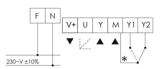
(\*) In order to use the floating control the only possible connection is between terminal M and Y1/Y2. Do not connect Y1/Y2 to phase (F) or neutral (N).
