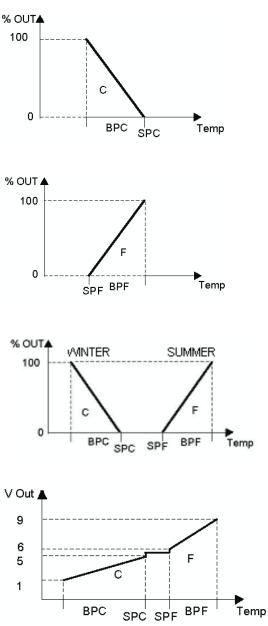
In this case, if a heating-Cooling sequence is required, the two actuators must be connected n parallel to the same output selecting the range 1 - 5 Vdc with <u>reverse</u> action for the actuator, which manages the heating channel, while for the actuator managing the Cooling channel, it is necessary to select the range 6 - 9 Vdc with <u>direct</u> action.
