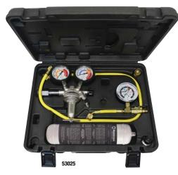
53025 PRESSURE TESTING REGULATOR KIT (France/Germany) 53002 Nitrogen Pressure Regulator, 48" Yellow Charging Hose (47482), Leak Testing Adapter (53042), R410a Straight Adapter 1/4 FL-M x 5/16 Swivel-F (90413), Regulator Adapter (53002-AD), 1 liter bottle of nitrogen (91150), Blow molded case (53000-PB)
